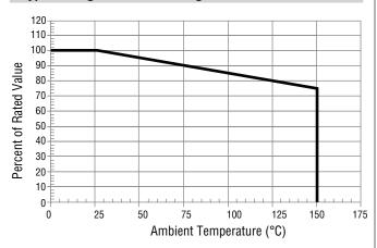
This graph shows the typical device surge current derating versus ambient temperature when subjected to the  $8/20~\mu s$  current waveform per the IEC 61000-4-5 specification. This device is not intended for continuous operation at temperatures above 125 °C.
