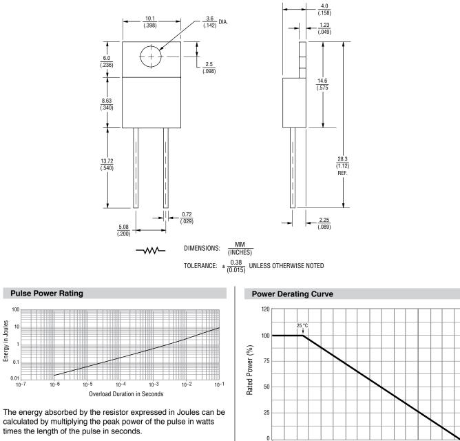
The energy should not exceed the limits shown in the graph. The overload voltage should not exceed 1.5 times the maximum
