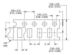
NOTES: TAPE MATERIAL IS PAPER. TAPE THICKNESS IS  $\frac{0.48\pm0.03}{(0.019\pm0.0012)}$  COVER TAPE ADHESION IS 40  $\pm$  15 GRAMS.
