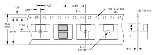
TOLERANCES: ±0.13 UNLESS OTHERWISE SPECIFIED DIMENSIONS: MILLIMETERS
