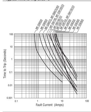
The Time to Trip curves represent typical performance of a device in a simulated application environment. Actual performance in specific customer applications may differ from these values due to the influence of other variables.
