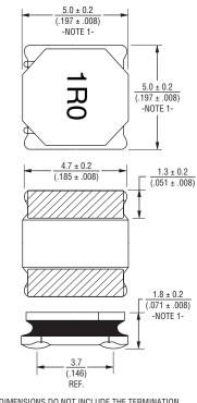
NOTE 1: DIMENSIONS DO NOT INCLUDE THE TERMINATION. FOR MAXIMUM OVERALL DIMENSIONS WITH TERMINATION, ADD 0.1 MM (.004 IN.).
