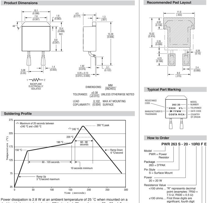
double-sided copper board using FR4 standard, 70  $\mu$ m of copper, 39 x 30 x 1.6 mm.
