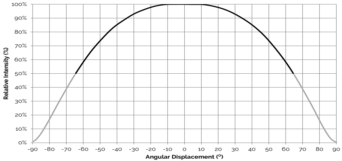
Figure 9: Typical Spatial Radiation Pattern
