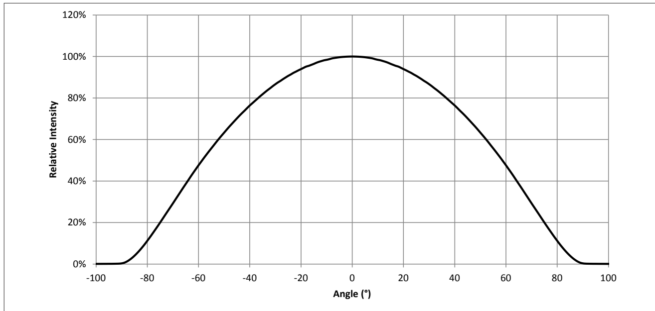
Figure 7: Typical Spatial Radiation Pattern
