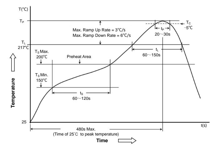
8.2 Classification of peak package body temperature (T<sub>P</sub>) 封装体峰值温度(T<sub>P</sub>)分类
