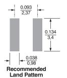
copper terminations, dimensions are for the mounted part. Dimensions before mounting can be an additional 0.005 inch / 0.13 mm.
