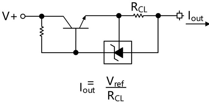
$$I_{out} = \frac{V_{ref}}{R_{CL}}$$
