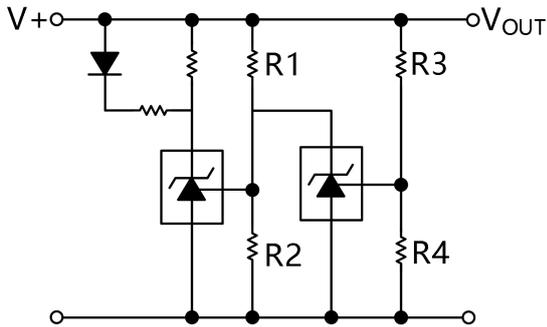
LED Indicator is 'on' when V+ is between the upper and lower limits.
