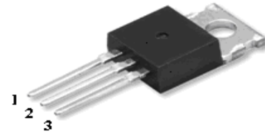
1.Gate 2. Drain 3. Source
