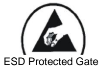
ESD Protected Gate
