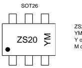
$\begin{array}{l} ZS20 = \mbox{Product Type Marking Code} \\ YM = \mbox{Date Code Marking} \\ Y \mbox{ or } \overline{Y} = \mbox{Year (ex: C = 2015)} \\ M \mbox{ or } \overline{M} = \mbox{Month (ex: 9 = September)} \end{array}$
