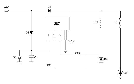
Note: The optional Capacitor C1 and Diode D3 are for power stabilization. C1 is recommended to be E-Cap., luF/25V; D3 is recommended to be Zener Diode, V<sub>z</sub>=27V. Which C1and D3 value need to be fine tuned to optimize design for different coils and power suppliers.
