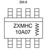
ZXMHC10A07 = Product Type Marking Code YWW = Date Code Marking Y or  $\overline{Y}$  = Last Digit of Year (ex: 5= 2015) WW or  $\overline{WW}$  = Week Code (01~53)
