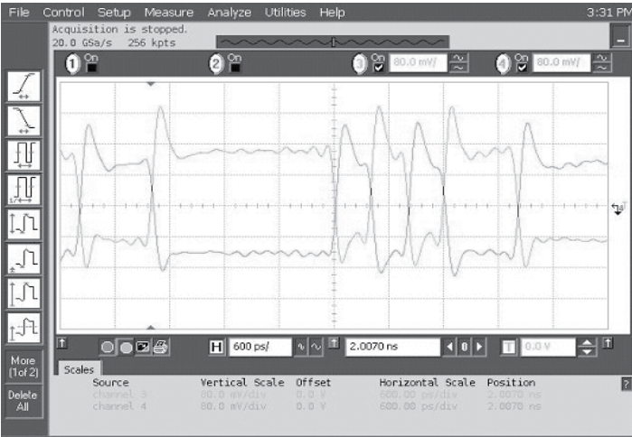
Data Waveforms, 3.0Gbps (left) & 6.0Gbps (right)
