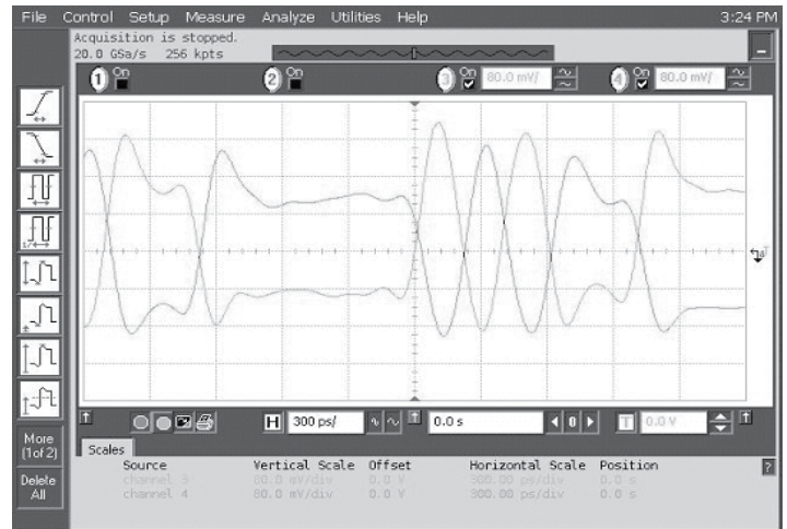
Data Waveforms, 3.0Gbps (left) & 6.0Gbps (right)
