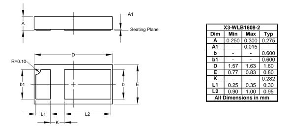
Note 7: Device side walls are electrically active bare silicon. Avoid contact of solder or flux on the side walls during the PCB assembly process.
