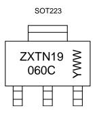
ZXTN19 060C = Product Type Marking Code YWW = Date Code Marking Y or  $\overline{Y}$  = Last Digit of Year (ex: 5= 2015) WW or  $\overline{W}W$  = Week Code (01~53)
