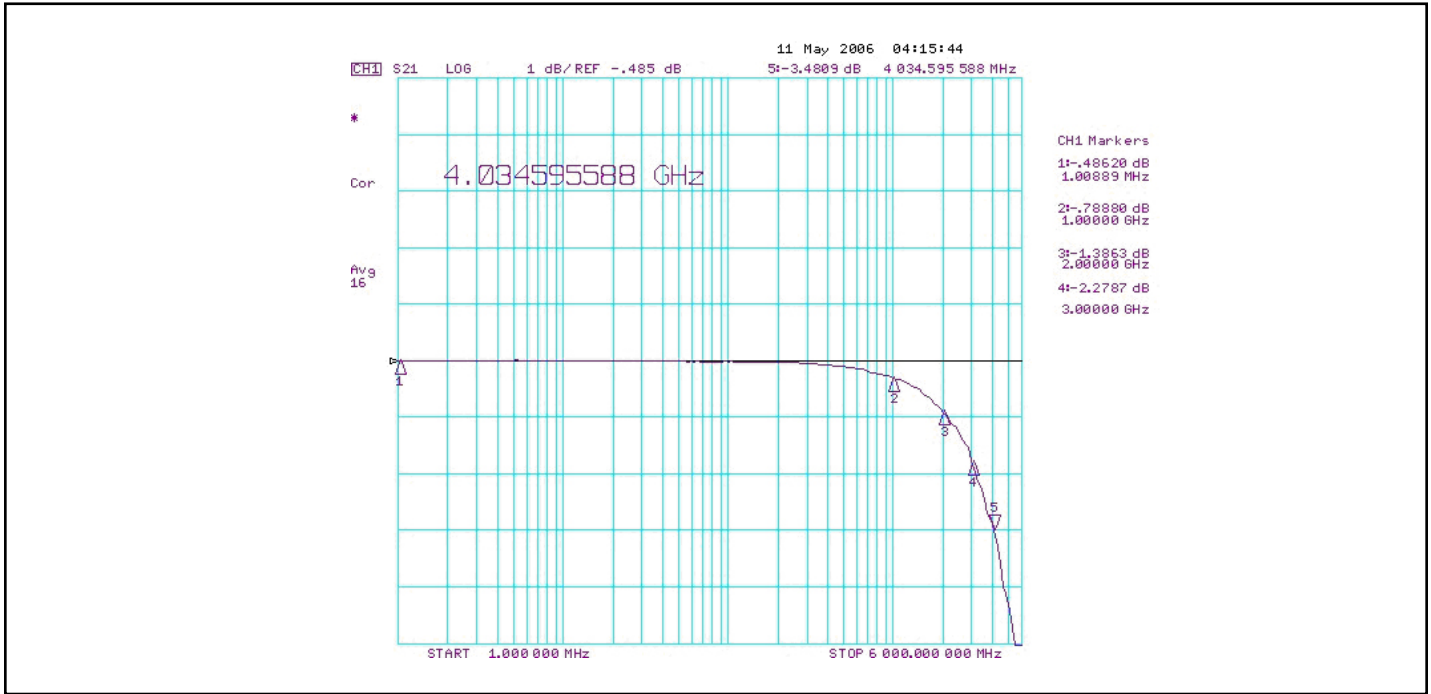
Fig 5: Typical Insertion Loss Plot from 1MHz to 6.0GHz, VDD=1.5V, 25C
