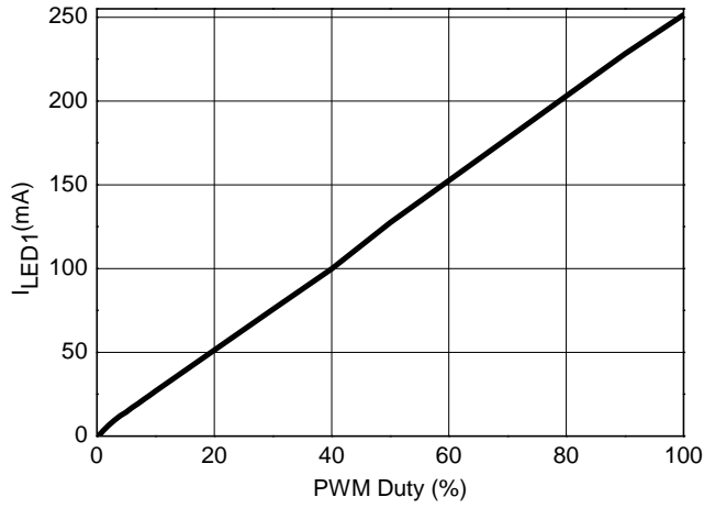
LED Current (AL1782) vs. PWM Duty (f=500Hz, 0~100%)
