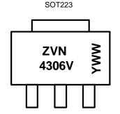
ZVN4306V = Product Type Marking Code YWW = Date Code Marking Y or  $\overline{Y}$  = Last Digit of Year (ex: 5= 2015) WW or  $\overline{WW}$  = Week Code (01~53)
