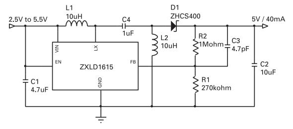
1 Cell Li-Ion to 5V Sepic Converter
