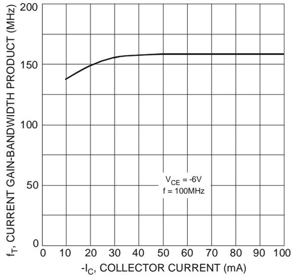
Figure 6 Typical Gain-Bandwidth Product vs. Collector Current
