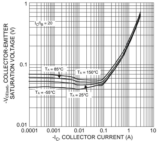
Figure 2 Typical Collector-Emitter Saturation Voltage vs. Collector Current
