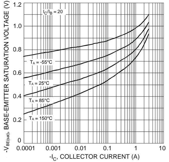
Figure 4 Typical Base-Emitter Saturation Voltage vs. Collector Current
