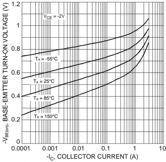
Figure 3 Typical Base-Emitter Turn-On Voltage vs. Collector Current
