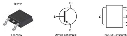
Pin Out Configuration Top view
