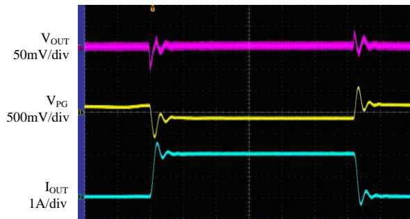
Load Transient (V CTRL =V EN =5V, V IN =2.2V, I OUT =0 to 2A)
