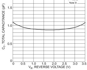
Figure 6 Typical Total Capacitance vs. Reverse Voltage
