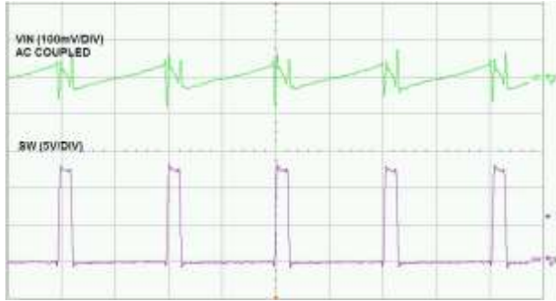
Time- 1µs/div Input Voltage Ripple
