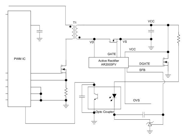
Secondary-side Synchronous Rectification
