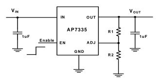
The output voltage is calculated by:
