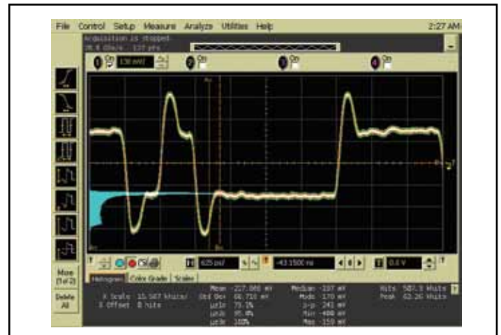
Output Waveform (400mV, 6dB pre-emphasis)
