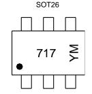
717 = Product Type Marking Code YM = Date Code Marking Y or  $\overline{Y}$  = Year (ex: C = 2015) M or  $\overline{M}$  = Month (ex: 9 = September)
