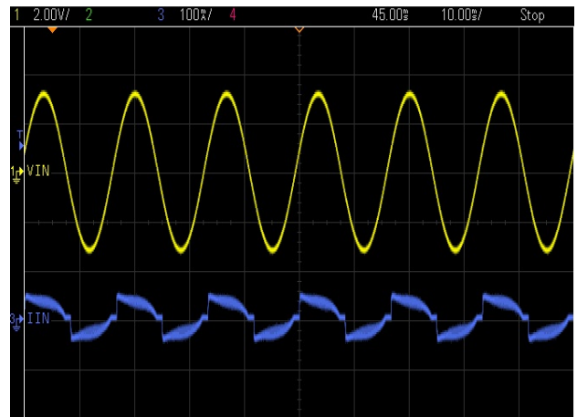
Figure 12. Input AC voltage vs. input AC current
