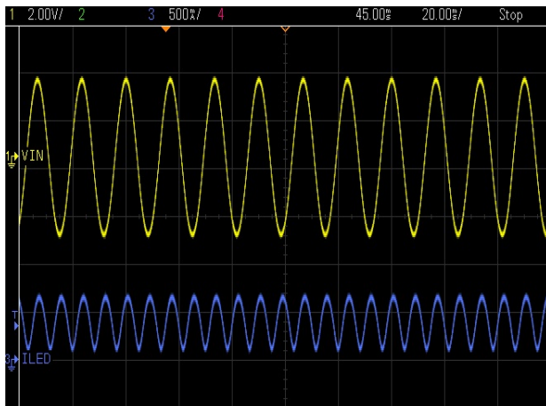
Figure 11. Input AC voltage vs. output current
