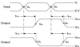
**Inverting and Non Inverting Outputs**
