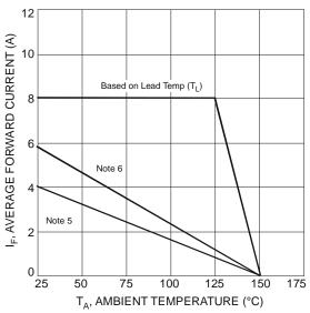
Fig. 6 Forward Current Derating Curve
