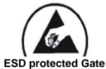
ESD protected Gate
