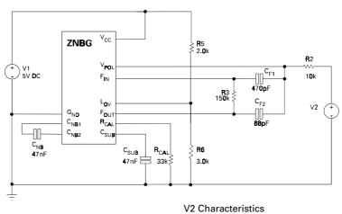
Type AC source Frequency 22kHz
