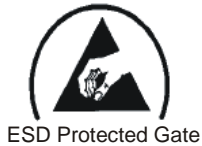
ESD Protected Gate
