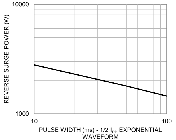
Fig. 4 Reverse Power Capability
