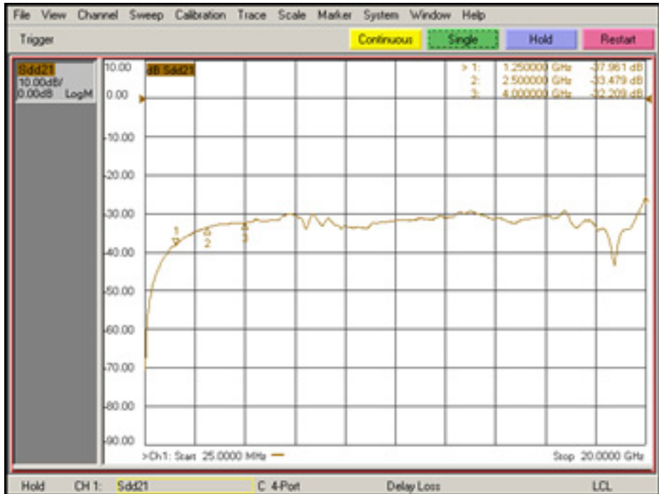
Fig 4. Differential Crosstalk – Super Speed
