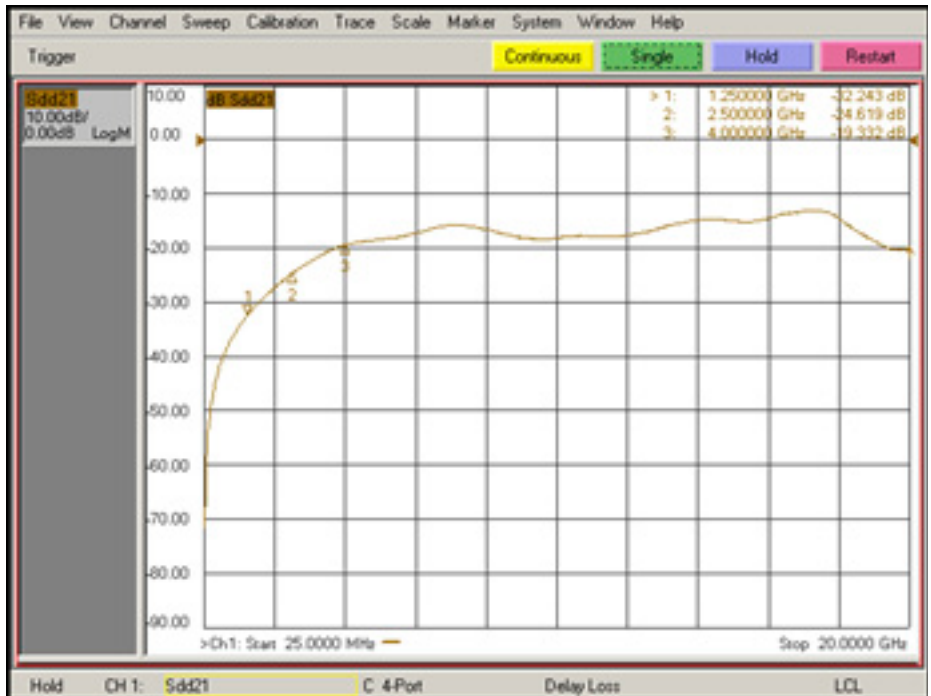
Fig 5. Differential Off Isolation – Super Speed
