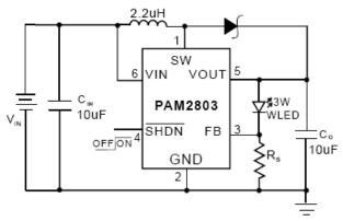
$I_{LED} = 750 \text{mA}, R_S = 0.127 \Omega$
