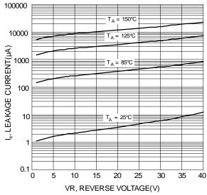
Figure 2 Typical Reverse Characteristics
