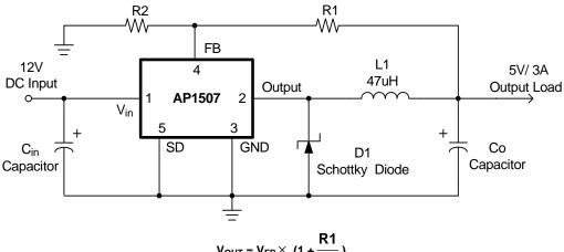
$$V_{OUT} = V_{FB} \times (1 + \frac{R1}{R2})$$
