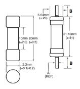
Dimension A (REF): 0.65 mm (0.5 A-6.3 A), 0.80 mm (8 A-10 A) Dimension B: For BK/packaging,  $38.1 \pm 0.38 \text{ mm}$ For TR2/ packaging, 15.8  $\pm$  2 mm
