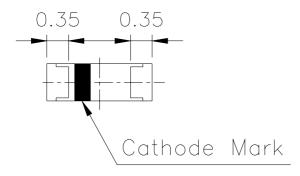
**Note:** The tolerances unless mentioned is  $\pm 0.1$ mm, Unit = mm
