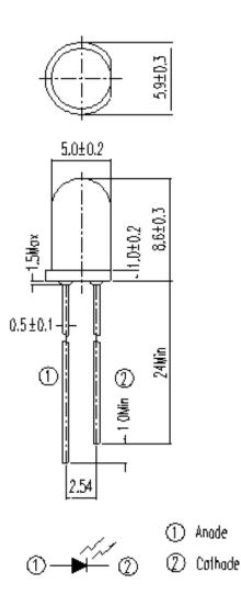
Note: Tolerances unless dimensions ±0.25mm
