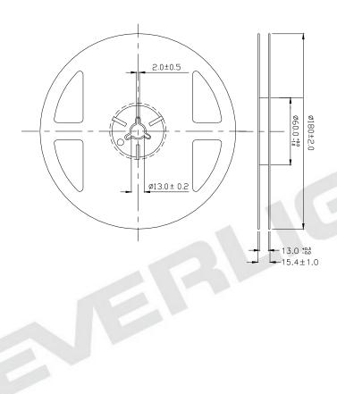
Note: The tolerances unless mentioned are ±0.1, unit=mm.
