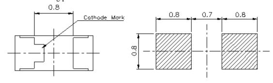
Note: Tolerances unless mentioned  $\pm 0.1$ mm. Unit = mm
