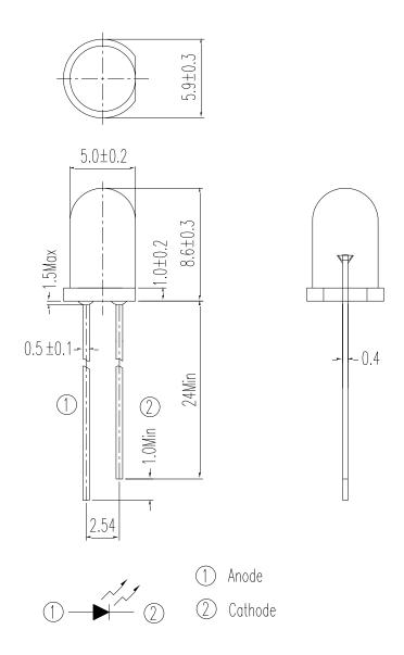
Note: Tolerances unless dimensions ±0.25mm
